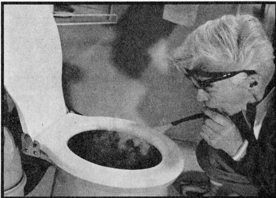
Rikart Lindstrom, the inventor, puffs smoke to show the powerful downdraught.
