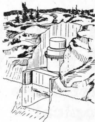
The Norwegian device, sitting in a gap blasted in the rock on the shore of an island off Bergen. A Norwegian artist's illustration of what it will be like.
