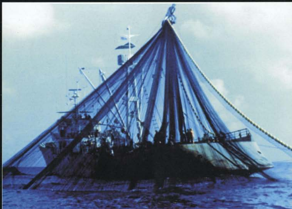
After closing the net and trapping the fish, the net is now run through the powerblock and then laid back on the stern of the fishing vessel.
