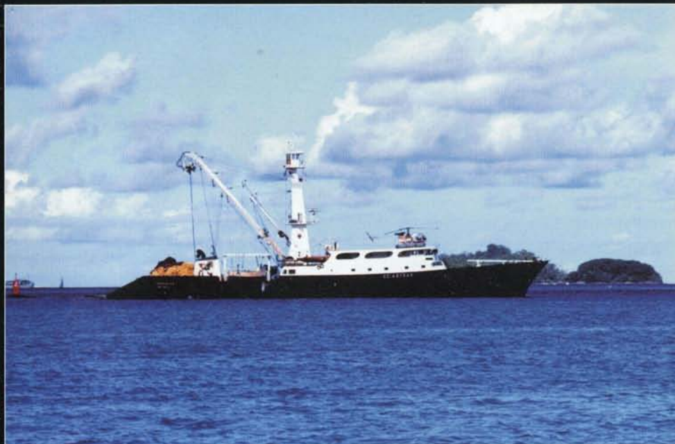
French tuna purse seiner F/V KERGUELEN at Mahe, Seychelles. Note helicopter on flying bridge. It is used to visually search for schools of tuna.
