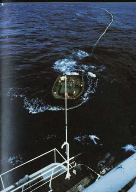
Encircling complete, the end of the net is brought back to the ship so that hauling in can proceed.
