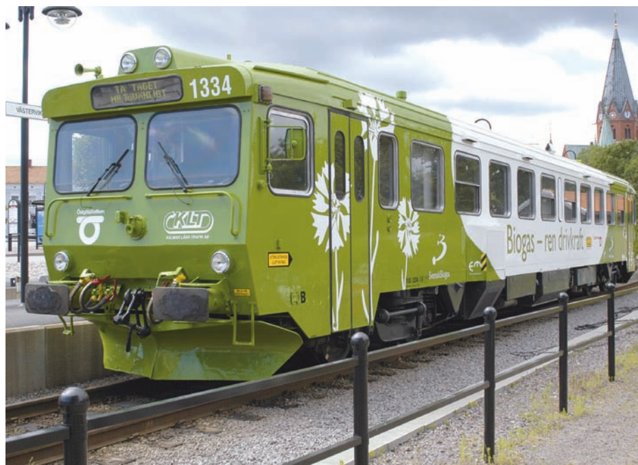
Last year Sweden unveiled the world's first biogas powered train. Driven by two biogas bus engines it can carry 54 passengers at 81mph, and run for 372 miles without refuelling
