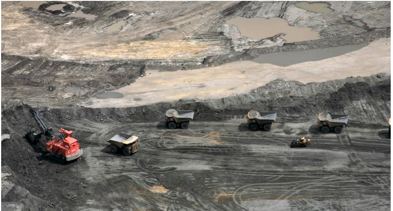
400-ton dumper trucks carry the bitumen rich sands from the mine face to refineries where it is heated with natural gas to drive off oil.
